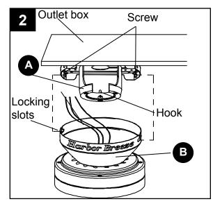
3. Install two non-slotted screws previously removed (Step 2, page 6) to canopy (B) and tighten securely.
