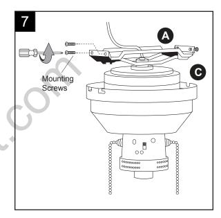
Attach the motor housing (C) to the mounting bracket
