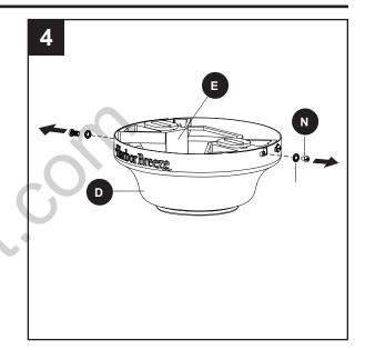
Attach mounting bracket (E) to outlet box (not included) using screws and washers provided with the outlet box.
