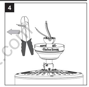
5. If you decided to cut back the lead wire in Step 4, strip 1/2 in. of insulation from the end of the white wire. Twist the stripped ends of each strand of wire within the insulation with pliers (not included). Repeat this step for black, blue and green wires.
