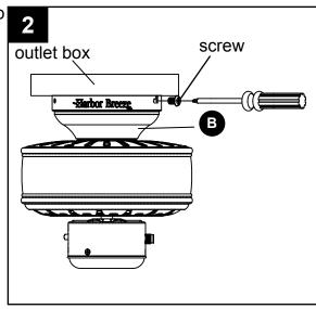
3. Directly align the locking slots of the canopy (B) with the two screws in the mounting bracket (A). Push up to engage the slots and turn clockwise to lock in place. Immediately tighten the two screws firmly. Install the two screws that were removed in previous step and tighten securely.
