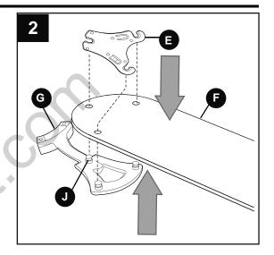
3. Place the plastic locking mechanism (E) on the opposite side of the blade (F) as the blade arm (G), refer to Fig. 2, with the *narrower* end of the plastic locking mechanism (E) toward the end of the blade (F) and against the blade screw (J) as shown in Fig. 3. [Please note the side of the plastic locking mechanism (E) indicating THIS SIDE UP.] Rotate plastic locking mechanism (E) to the left (counterclockwise) to lock plastic locking mechanism (E) into place.
