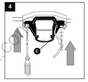
Remove motor screws (I) and lock washers (K) from underside of motor. [If there are plastic motor blocks installed with the motor screws (I) and lock washers (K), discard the plastic motor blocks.]
