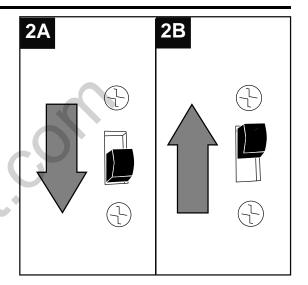
2C. **IMPORTANT**: Reverse switch must be set either *completely UP* or *completely DOWN* for fan to function. If the reverse switch is set in the *middle* position (Fig. 2C), fan will not operate.
