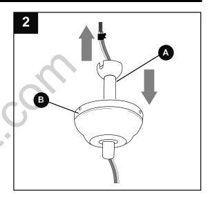
Slip downrod (A) into motor housing yoke, align holes and re-install pin (M) and clip (N).
