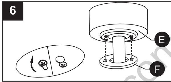
6. Loosen the two shoulder screws without fully removing the hanger bracket (A). Assemble canopy (E) by rotating keyhole slot in canopy over shoulder screws in hanger bracket (A). Tighten shoulder screws. Securely attach and tighten the canopy hole cover (F) over the shoulder screws in the hanger bracket (A) utilizing the keyhole slot twist-lock feature.
