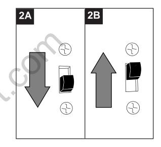
2C. **IMPORTANT**: Reverse switch must be set either *completely UP* or *completely DOWN* for fan to function. If the reverse switch is set in the *middle* position, fan will not operate.
