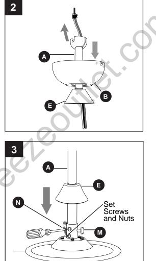
Slip downrod (A) into yoke, align holes and re-install pin (M) and clip (N). Tighten set screws and then tighten nuts on the set screws. Slide yoke cover (E) down until it rests on top of motor housing (D).
